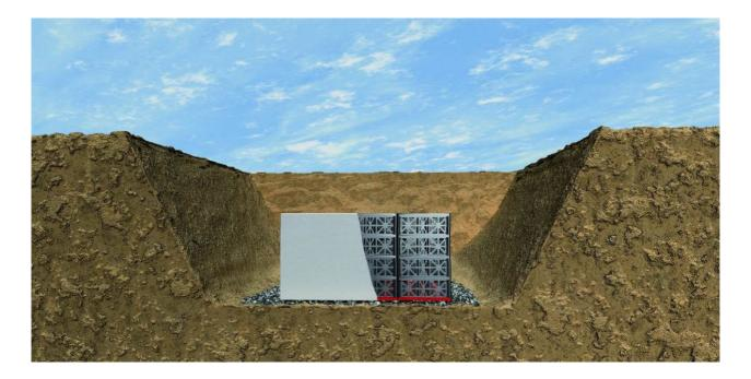
The excavation must also be designed in accordance with "Excavation pits and trenches" or similar standards. In particular, this includes the slope angle that has to be selected depending on the soil type for depths of 1.25 m (4'-1.2").
