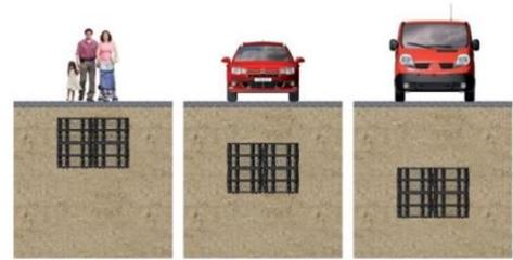
The resulting information determines the minimum and maximum cover depth and the maximum excavation depth. Table 1 shows the parameters for the different applications.
