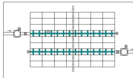
The design of the RAINBOX® 3S crate makes it possible to pass a camera through for inspection purposes.
